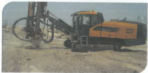
WET DRILLING PLUS DUST COLLECTOR
